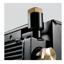
Temperature-controlled bypass valve Integrated Allows the oil to bypass the cooler matrix if the pressure drop is higher than 2,2 bar or less than the chosen temperature. The bypass closes when the oil temperature increases. Different closing temperatures available. Available for singlepass or two-pass matrix design
